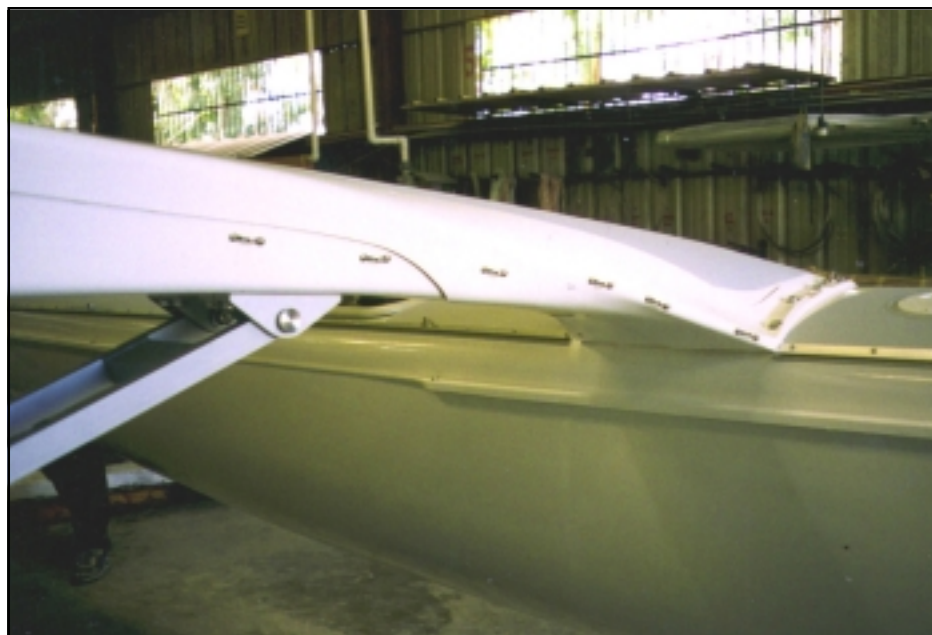
The latest F-28 Fwd. Beam cover which eliminates the forward join flange.
