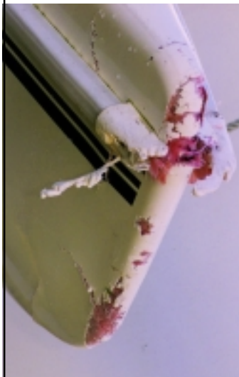
If there is this much bow damage (F-31 float Bow)
